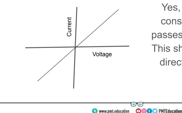
Yes, as the line has a constant gradient and passes through the origin. This shows that voltage is directly proportional to current.
