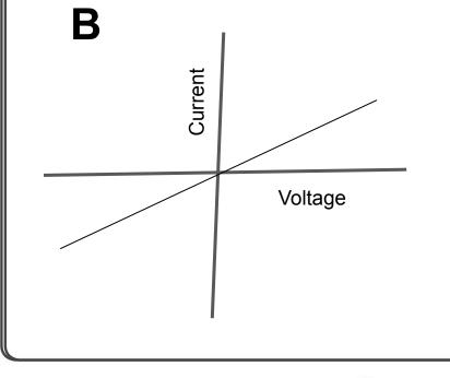
B has a shallower gradient, and as the gradient=1/R, a smaller value for the gradient = a
